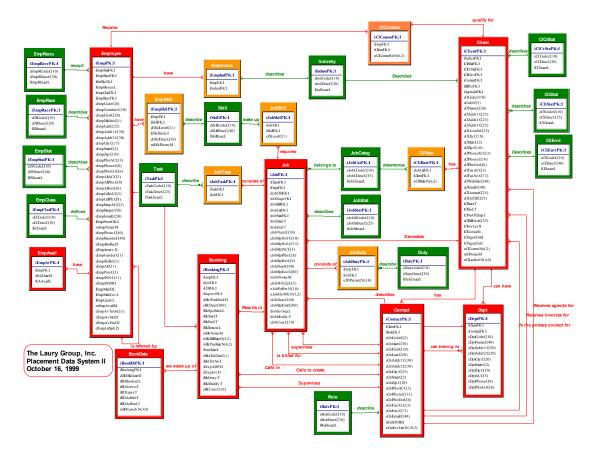
Figure 7: An Entity-Relationship diagram for a moderately complex application. For ease of presentation, the primary tables are in red, many-to-many tables in orange, and lookup tables in green.
